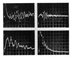
Fig. 3. Brain-implanted hydrophone responses to pulsed microwave irradiation in the cat (left) and guinea pig (right) at 5.655 GHz (top) and 2.450 GHz (bottom). Horizontal scale was 20  $\mu$ s/div. Vertical scales were 20  $\mu$ V/div for the cat; 100 and 200  $\mu$ V/div for the guinea pig at 2.450 and 5.655 GHz, respectively.
